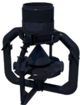
The innovative nozzle design is shaped to provide a square spray pattern, thereby uniformly wetting the entire fill media. This improves tower performance and reduces the likelihood of scaling due to the occurrence of dry regions
