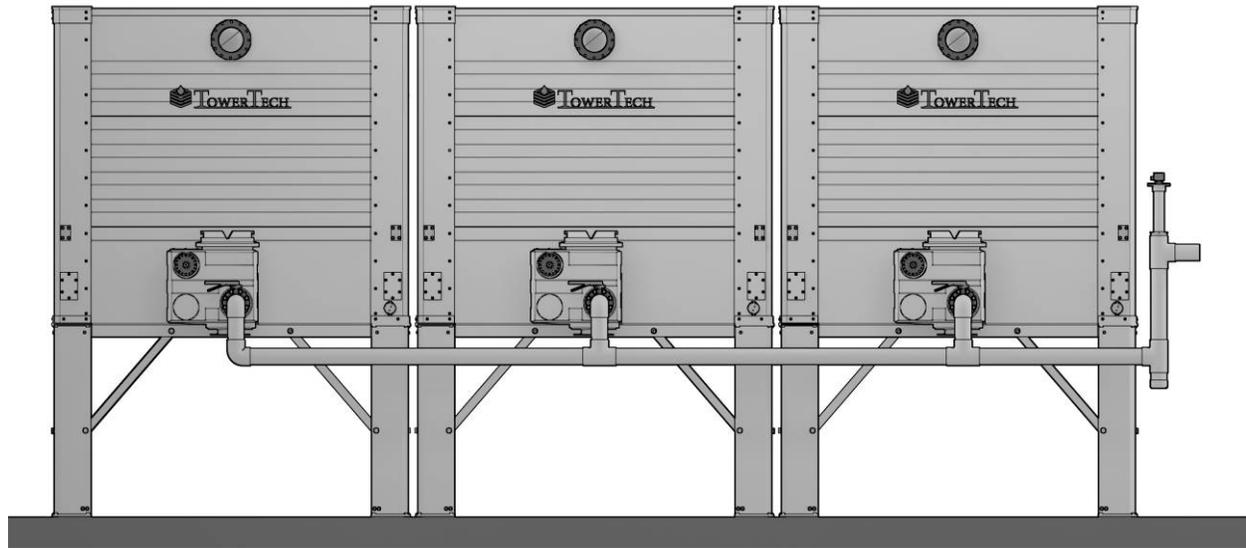
**Note:** Keep all vents clear and open. Stand pipes must be heat traced and insulated in cold climates.
