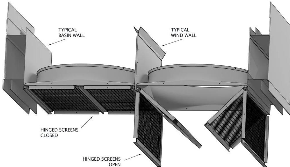
*Figure 55B – Opening Split Screen Fan Guard*
