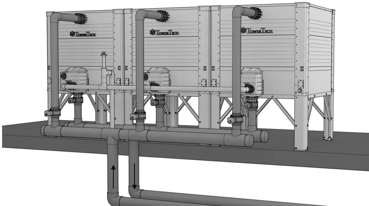
*Figure 21 – Multi-Tower Layout and Piping Recommendations*
