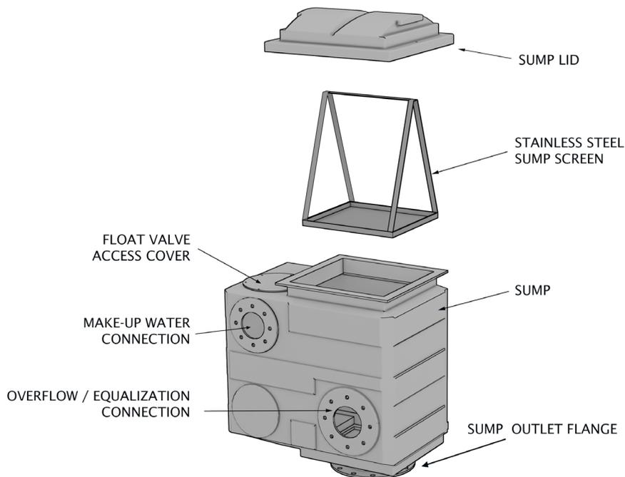
Figure 57 – Sump Layout, Sump Screen Detail
