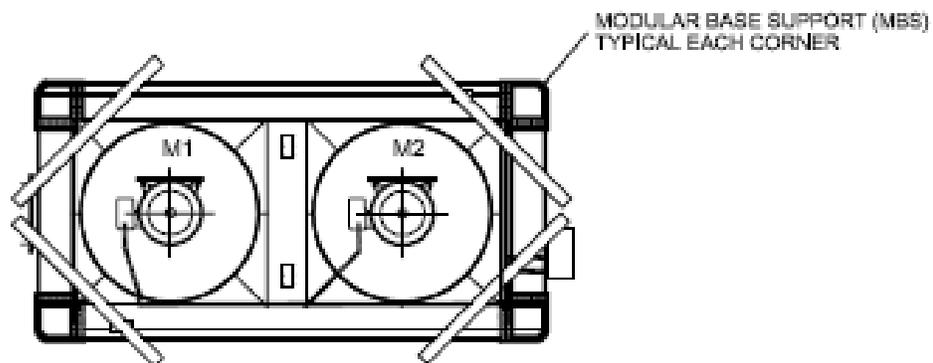
Figure 33 – Cribbing Detail
