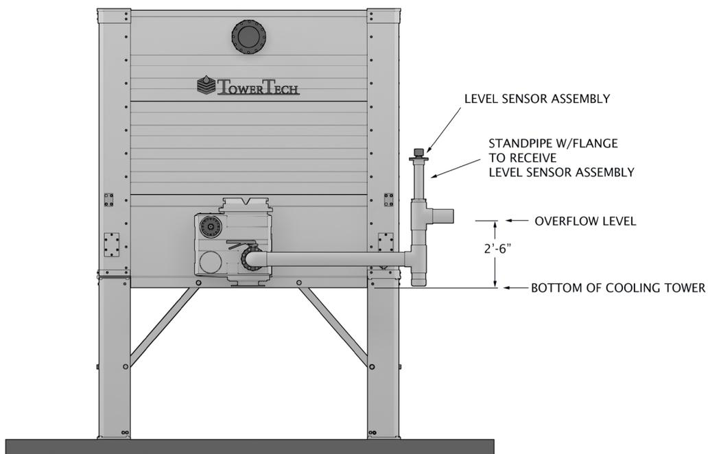
Figure 18A – Ultrasonic Liquid Level Sensor Location
