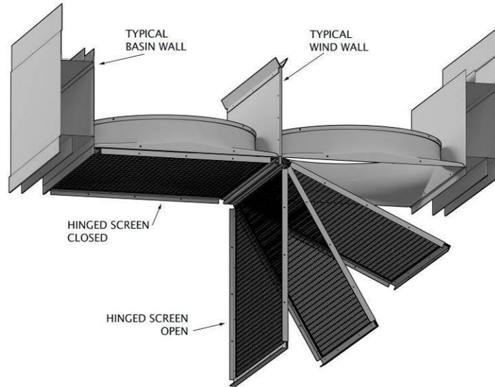
*Figure 55A – Opening Full Screen Fan Guard*
