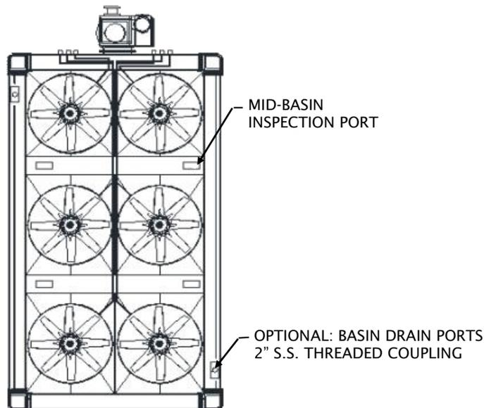
Figure 47 – Mid-Basin Inspection Ports (6-fan tower module shown)
