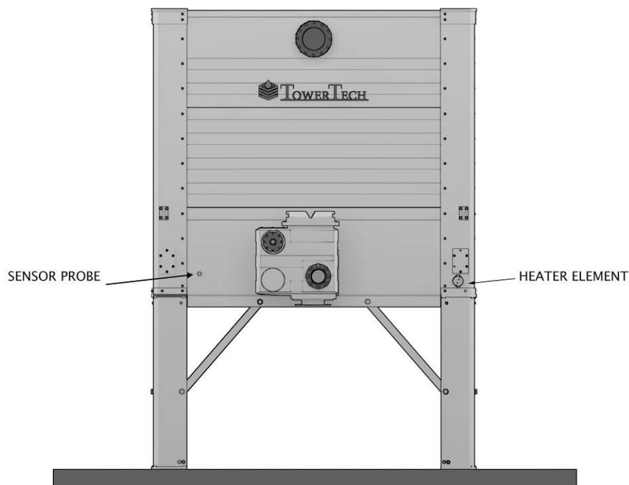
Figure 17 – Immersion Basin Heater and Sensor Probe Location
