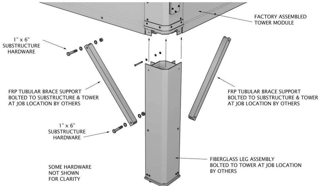
Figure 14 – Tower Sub-Structure
