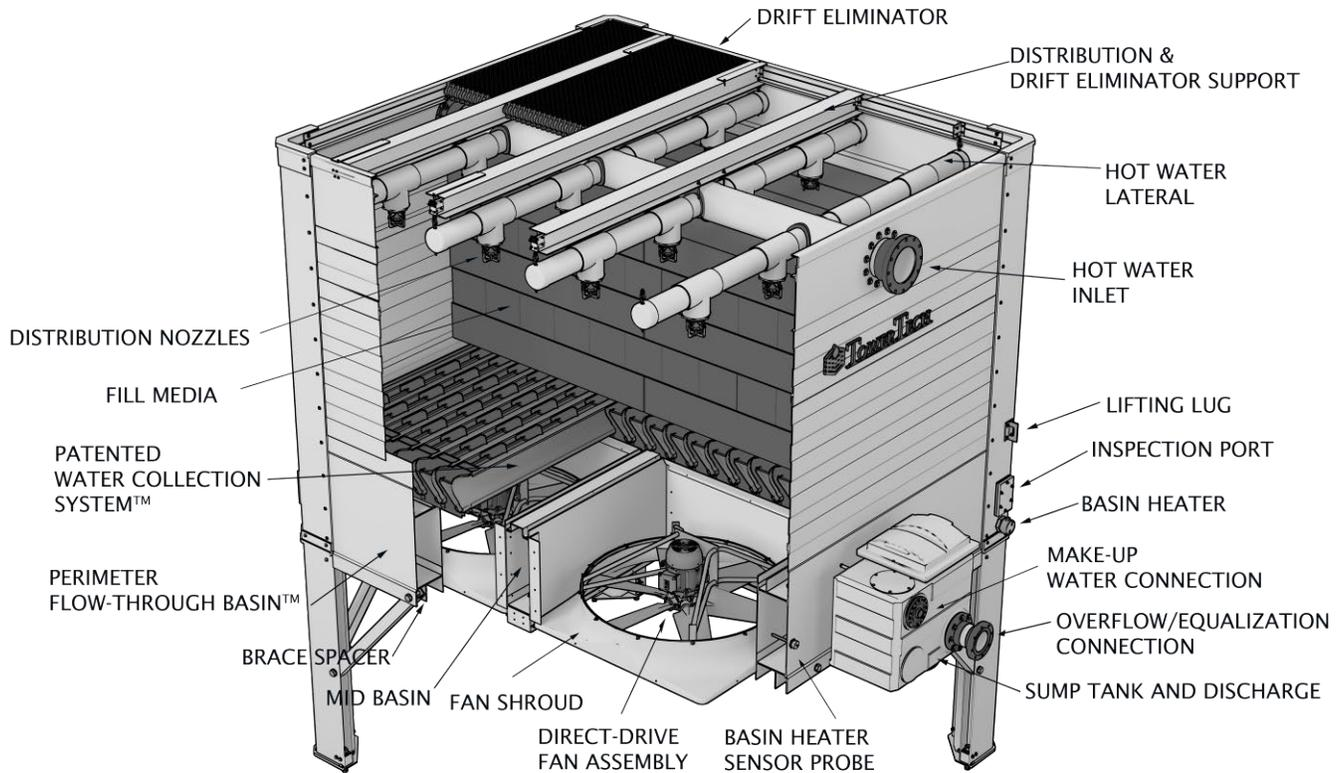
Figure 1 - TTXR 3-D Cut-Away View
