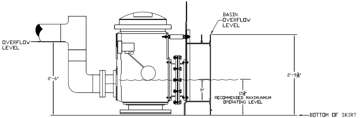
Figure 19B – Sump Detail With Equalization/Overflow Pipe (No Ultrasonic Level Sensor)
