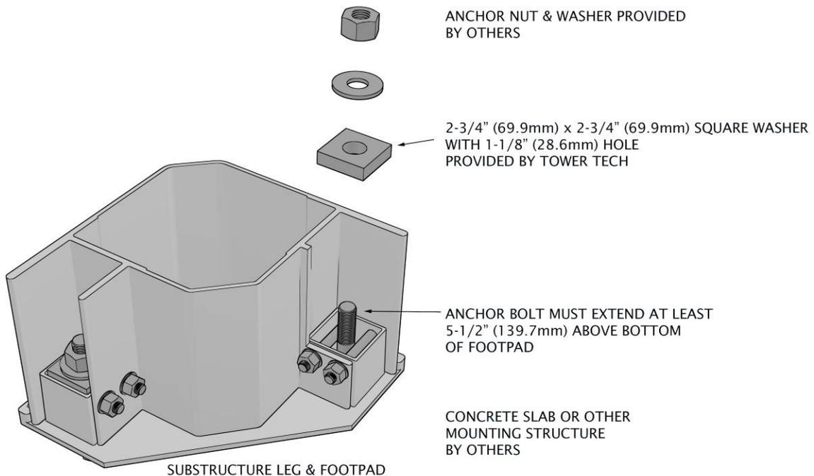
Figure 31 – Installation Detail for Sub-Structure Footpad
