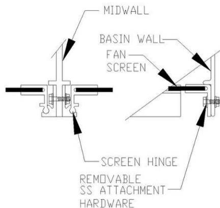
Figure 54 – Close-Up: Fan Guard Hardware
