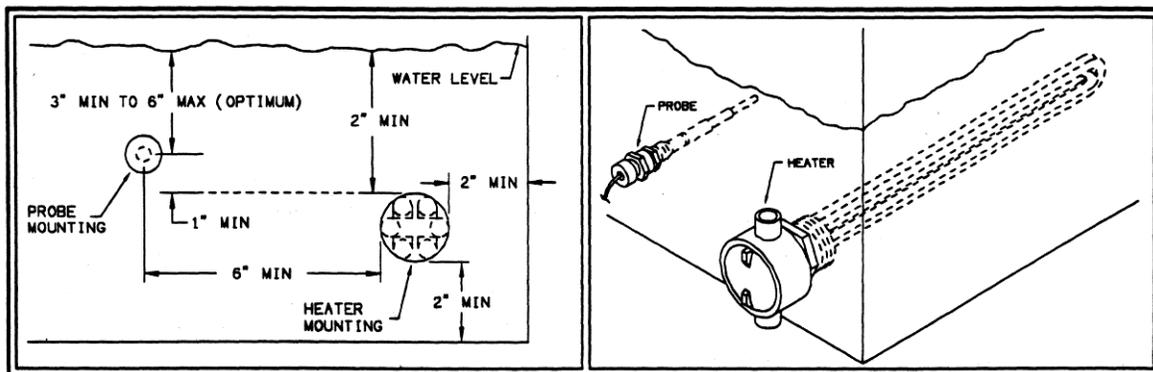
Figure 49 – Location of Basin Heater Probe & Element
