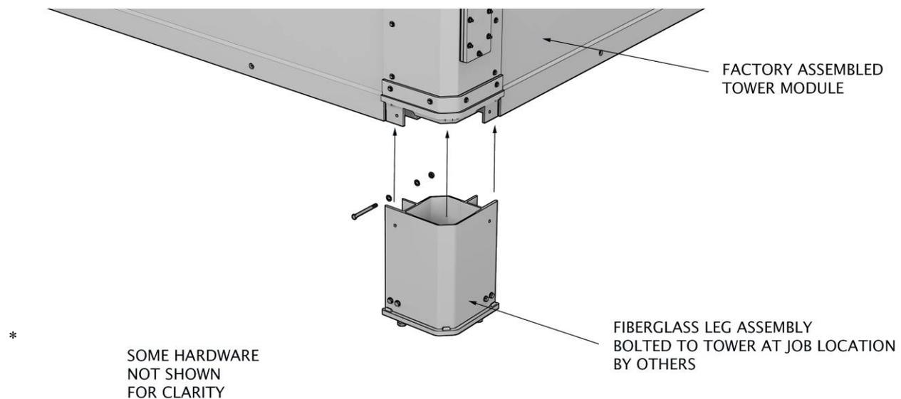
Figure 30 – Installation Detail for 1' Sub-Structure
