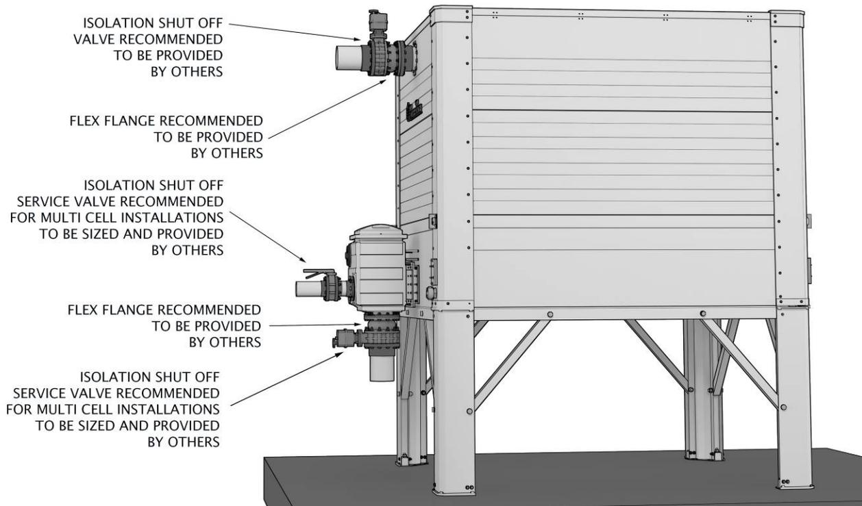
Figure 37 – Connection Flexible Flanges & Flow Control Valves
