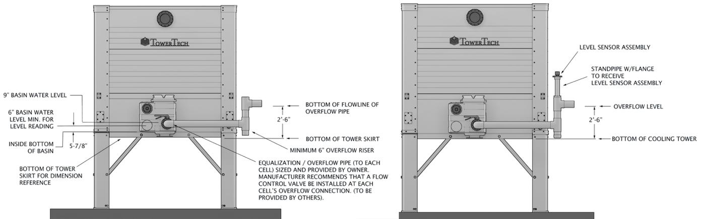
Figure 39A – Typical Overflow/Equalization Pipe
