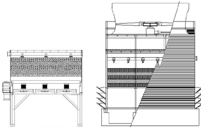
*Figure 3 – TTXR versus Conventional Induced-Draft Counter-Flow Tower*
