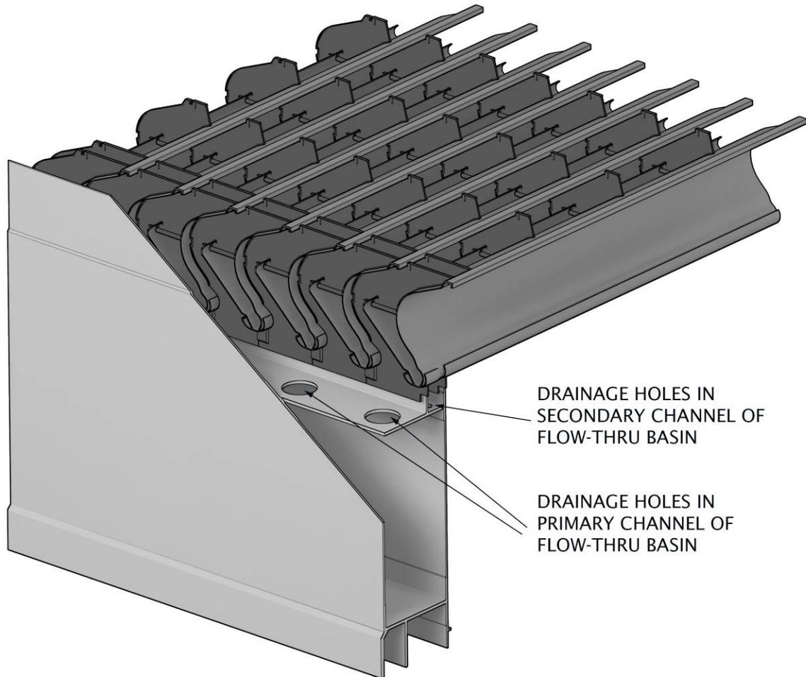
Figure 60 – Flow-Thru Basin Drainage (Perimeter Basin Wall)
